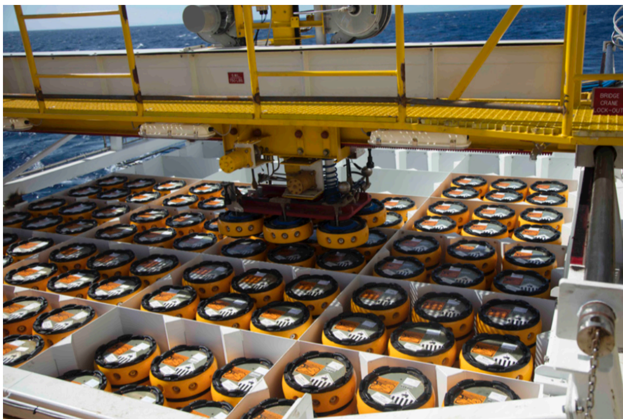
Figure 7: Main picture: Automated deployment of ocean bottom nodes (Mageis Fairfield Nodal ZXPLR® system) in a deepwater setting (Image from Mageis Fairfield).
